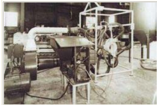
Fig. 1. In 1960, when there was no commercially available equipment to apply powder to pipe, 3M built this pipe-coating machine to apply its Scotchkote 101 epoxy powder. Photo courtesy Rupert F. Strobel, 3M Co.
