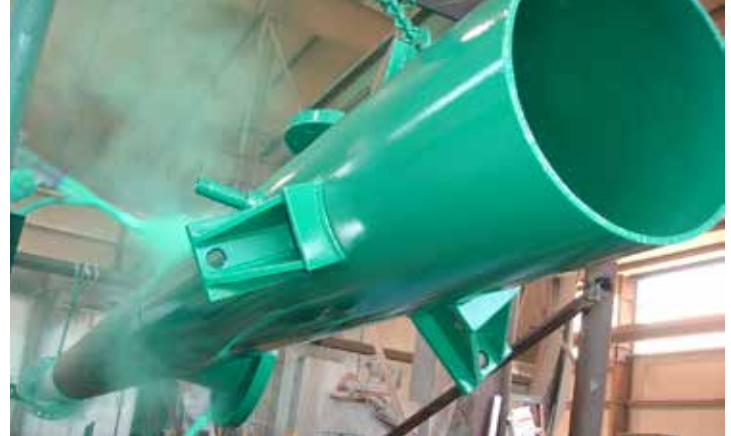
Custom pipe being coated to AWWA's C213 specification
