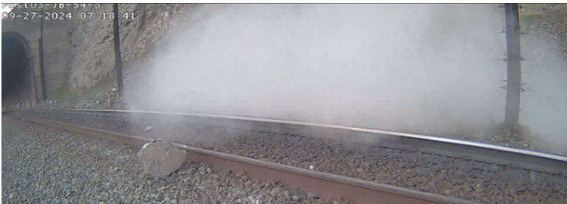
Fig. 1. Qualifying Rockfall Event Captured by Rockfall Monitoring, Missed by Slide Fence
