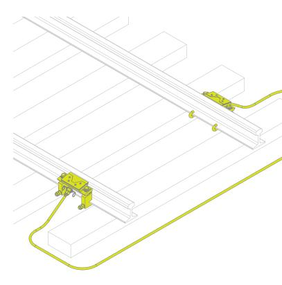
The TGA3 is typically installed at the approach and exit to stations, signals and on track inclines. The TGA3 reliably deploys the required amount of traction enhancing material to the top of rails via application bars.
