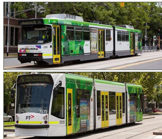
Figure 4. Top: B Class Tram (High Floor), Bottom: D Class Tram (Low Floor)
