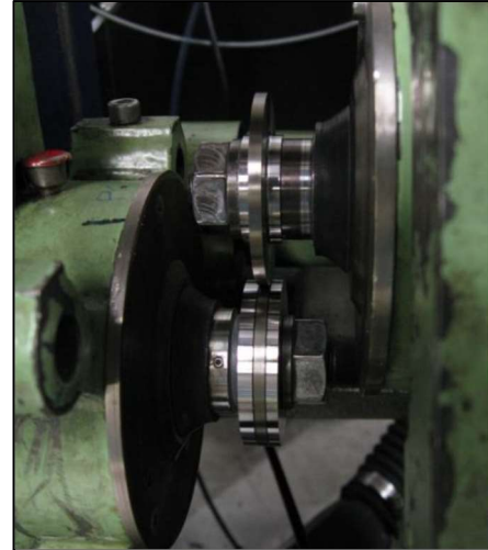
FIGURE 2: Twin disk testing of traditional petroleum grease and premium synthetic.
