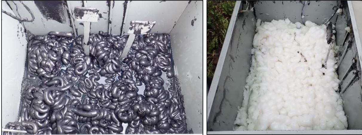
FIGURE 13: Comparison of oil separation of traditional petroleum grease (left) versus premium synthetic (right).
