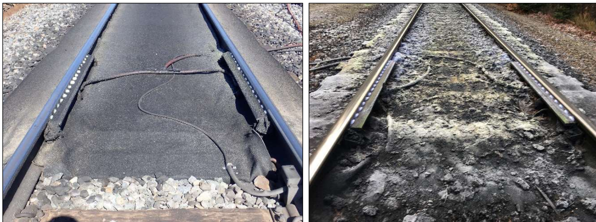
FIGURE 12: Reduced port clogging recorded in heavy sanding areas with premium synthetic grease
