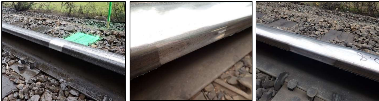
FIGURE 10: MP10.8 4°45" left hand curve inspection: traditional petroleum-based June 2018 (left), premium synthetic August 2018 (center) and October 2018 (right).
