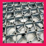
The supporting mosaic grids are made from electro galvanised, die cast, zinc aluminium alloy. The grids are precision cast to provide support of the mosaic tiles and their components. Mosaic grids are assembled to form the mimic structure and are consolidated via a perimeter extruded aluminium bezel. High accuracy die cast grids characterise the Subklew system as being the market leader.
