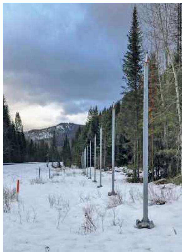
Each gateway can currently monitor up to 20 tags, spaced at broadly 10 m intervals. A typical installation with three or four gateways can monitor around 600 m.
