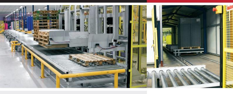
Once the sub assembly operations have been completed the finished totes are stacked on empty pallets at the rear of the assembly areas. These pallets are replenished by powered roller conveyor from an automated pallet dispenser. The full pallets are sent by transfer device via the conveyor to the second shuttle car for their onward journey into the warehouse.
