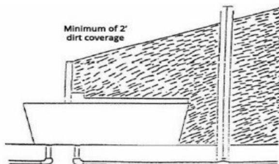
Figure 2. Bank or Pond Dam Installation
