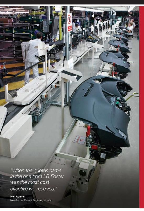
Leicester based LB Foster Materials Handling has recently completed the installation of a continuously moving, inverted monorail conveyor for a dashboard sub assembly line at Honda's UK manufacturing plant in Swindon.
